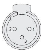
DMX-OUTPUT XLR mounting-sockets (rear view)
